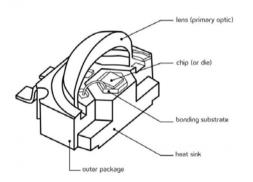
Fig.3: Typical LED package. [2]
