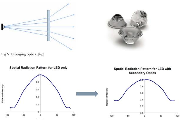
Fig.7: Change in light beam width using diverging optics. [4]
