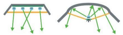
Fig.10: Change in light beam width using diverging optics. [4]
