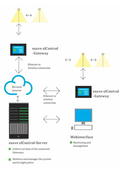
Figure 7: esave slControl – street light management solution
