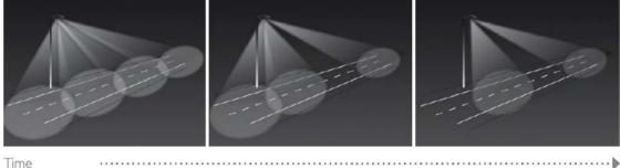
Fig.12: Dimming strategy: Multi-layer and Multi-spot. [1]
