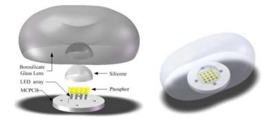
Fig.4: Primary optical system of LED chip array module. [3]
