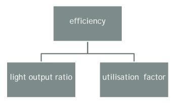
The Light output ratio (L.O.R) is a necessary property to define the efficiency of a luminaire. As the L.O.R approaches to one, more light will come out of the luminaire. This factor is the ratio between the luminous flux produced by the lamp to the luminous flux coming out of the luminaire. The differences between the two are termed as losses. Losses can be:
