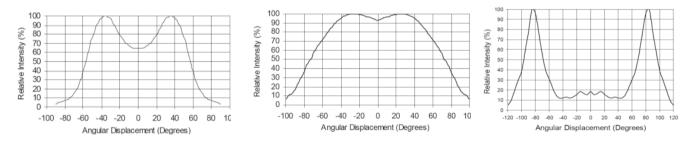
Fig.1: a. Batwing; b. Lambertian; c. Side-emitting. [1]
