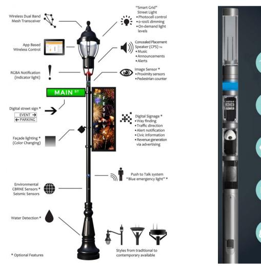
Fig.13: Example of multi-functional luminaires; Intellistreets. [18]
