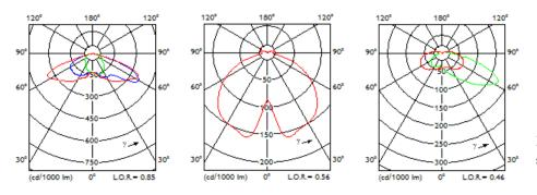
Fig.2: Typical light distributions in street lighting applications. [1]
