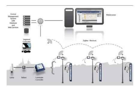
Figure 2: Princips of function of a wireless controle system [28]
